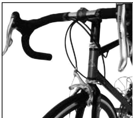
Fully Lugged Classic Road Bike With Full Internal Cables and Stainless Head Badge
