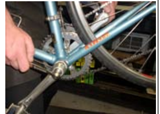
Jeremy having way too much fun installing a new bottom bracket into a 25 year old Rodriguez bicycle. This bike looks great, and was back on the road a day or 2 after the customer brought it in for service. Thanks to the ISO commission of the 1970's, this bicycle will probably be on the road another 50 years or more.
