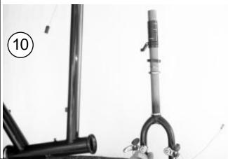
10.) Now put of the headset parts, spacers and the cable hanger back onto the fork in the order that they would be if they were on the bike. This helps you remember how things go back together during reassembly. Remember to put the headset adjusting cap and bolt back on to keep everything from falling off.
