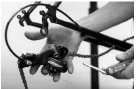
**<u>Do not</u>** disconnect the cable. The derailleur can just hang from the bike section.
