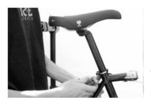
Remove the seat using the appropriate Allen wrench. Make sure to note your seat height. Some people like to put a scratch on the seat post, others will use a piece of electrical tape.
