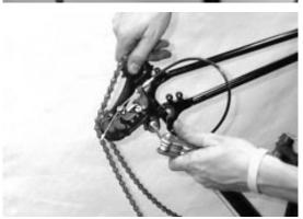
REINSTALLATION - There is a tab on the bike frame and a tab on the derailleur that need to be in the right position when you reinstall the derailleur. Make sure to 'rotate' the derailleur towards the back of the bike while you tightened the mounting bolt. Otherwise, you can break the tab off of the derailleur and it won't work right.
