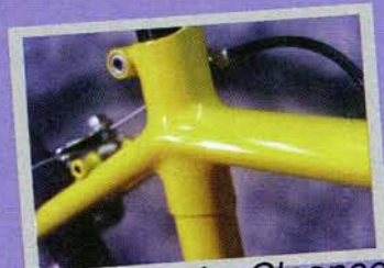
Sample of a Cleaned & Polished Weld
